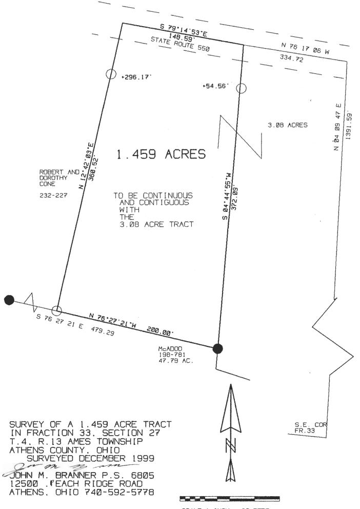
SCALE 1 INCH - 60 FEET O = IRON PIN SET • = IRON PIN FOUND BEARINGS BASED ON PREVIOUS SURVEY
