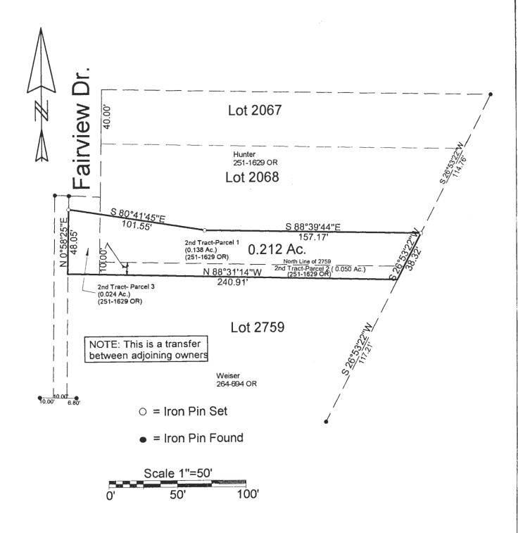
CERTIFICATION: WE HEREBY CERTIFY THAT THIS PLAT OF A MORTGAGE LOCATION SURVEY WAS PREPARED FROM ACTUAL FIELD MEASUREMENTS IN ACCORDANCE WITH CHAPTER 4733-38, OHIO ADMINISTRATIVE CODE, AND IS NOT A BOUNDARY SURVEY PURSUANT TO CHAPTER 4733-37 OF SAID CODE.
