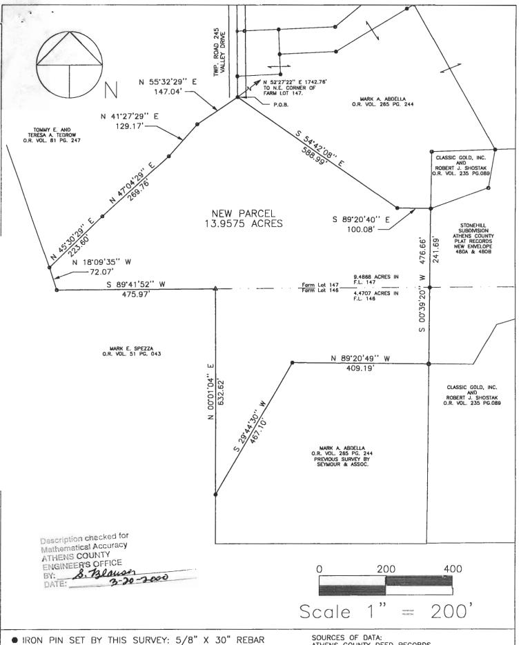
IRON PIN SET BY THIS SURVEY: 5/8" X 30" REBAR W/PLASTIC I.D. CAP: E. TRIPLETT S-6766.
