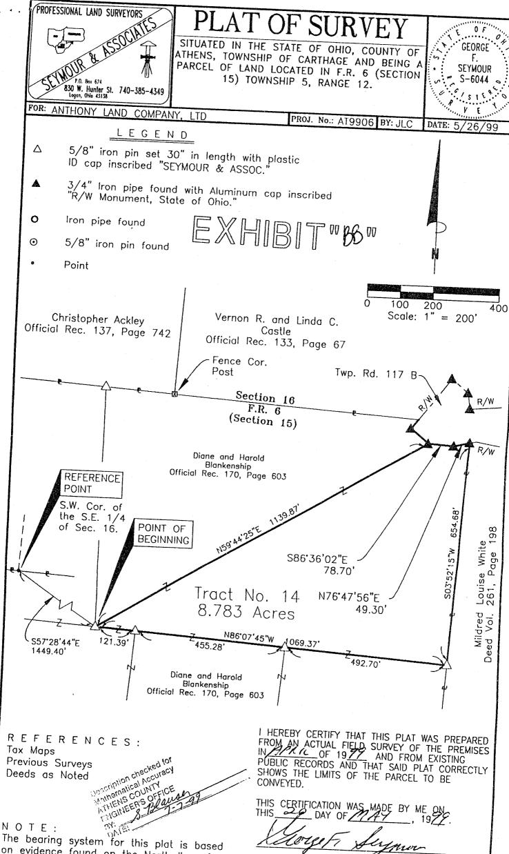
on evidence found on the North line of Section 15 and bears S 86° 27' 46" E and is for the determination of angles only.
