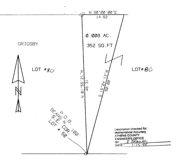
NOTE: THIS SURVEY WAS CONDUCTED TO ESTABLISH AN AGREED LINE BETWEEN EXISTING CURRENT OWNERS IN ORDER TO RESOLVE DESCREPANCY IN ADJOINING DEEDS CAUSING AN OVERLAP. THE ABOVE ATTACHED TRACT IS TO BE CONTINUOUS AND CONTIGUOUS WITH LOT
