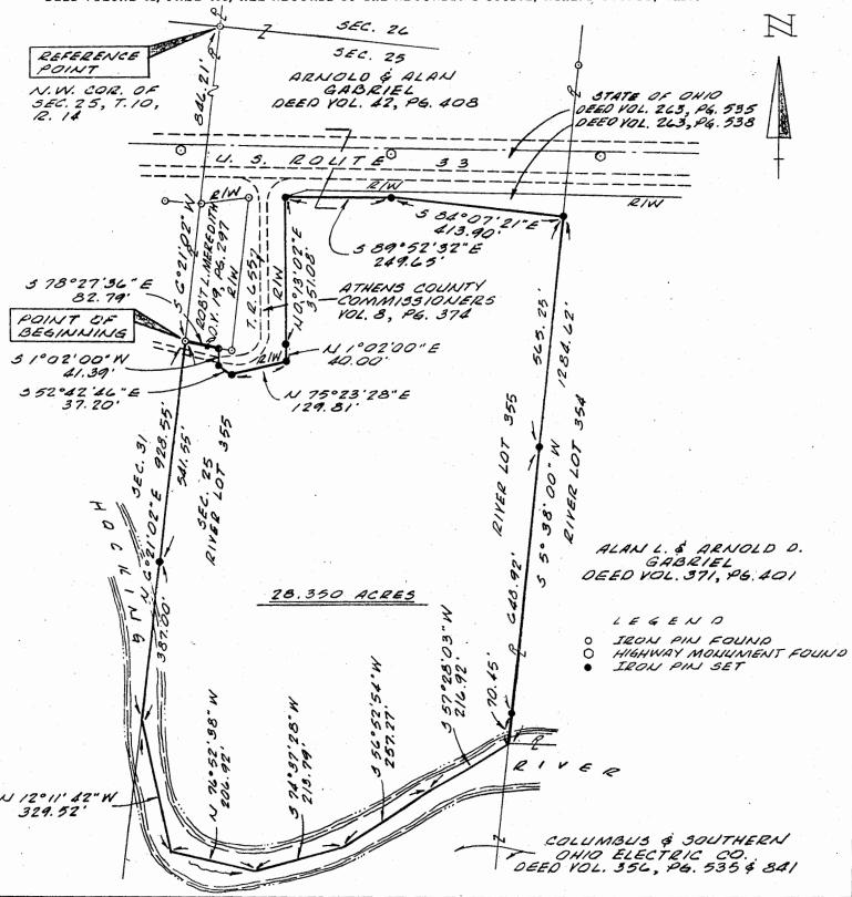
The bearing system for this plat is based on the centerline of U.S. 33 as being S  $88^{\circ}$  58' 00'' E as delineated upon Right of Way Plan "ATH-33-5.48".
