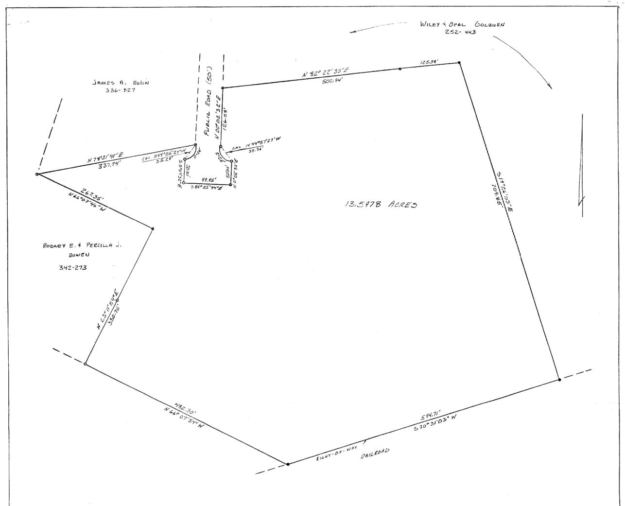
• = IRON PIN SET • = IRON PIN FOUND SCALE: 1"=100'
