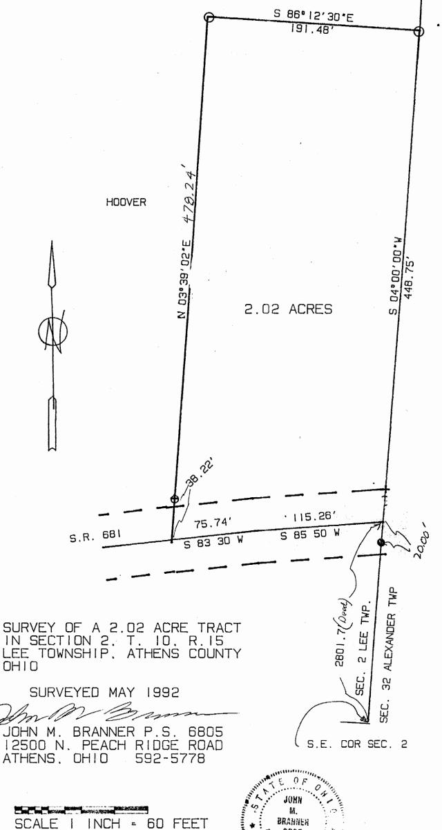
SCALE | INCH = 60 FEET O= IRON PIN SET O= IRON PIN FOUND
