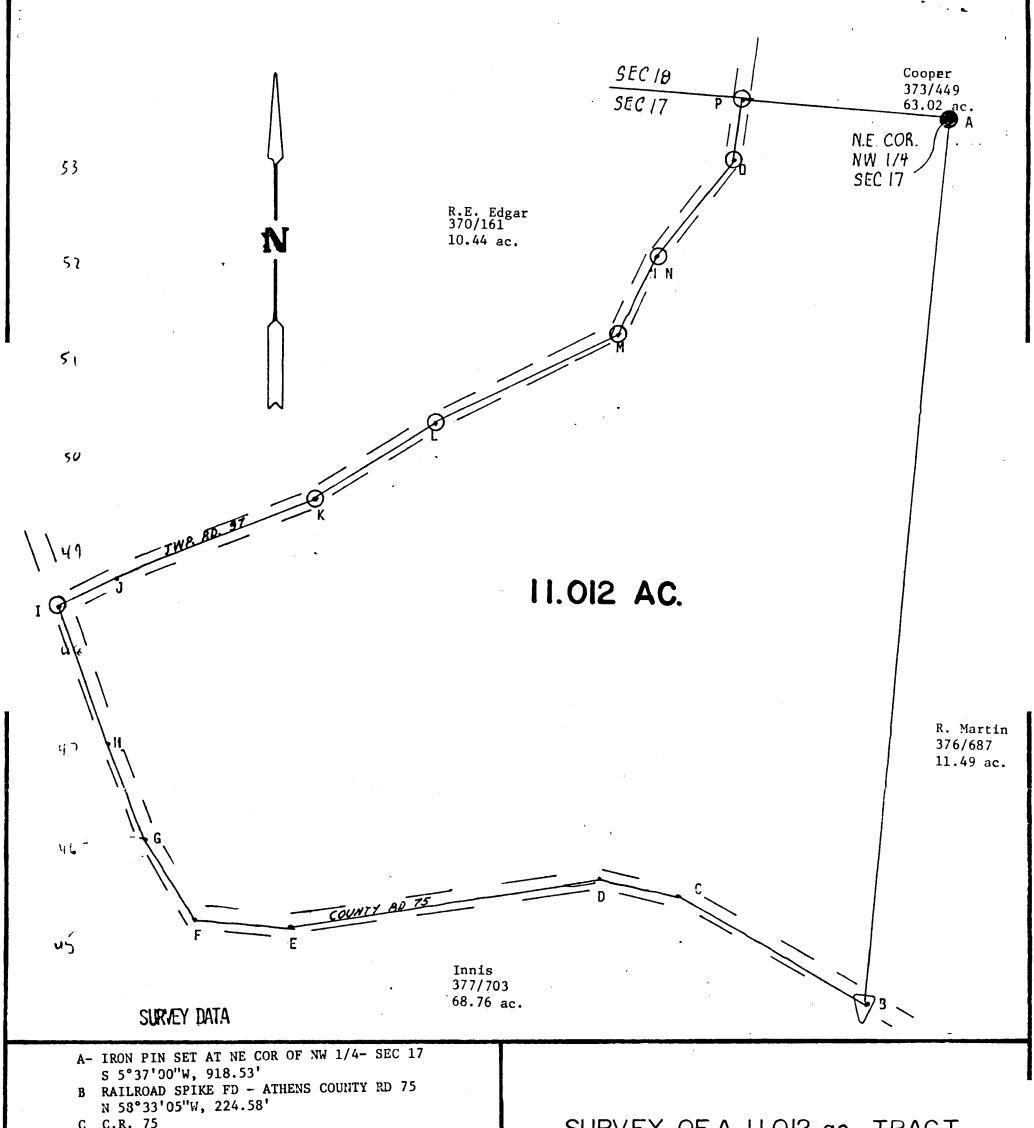
C.R. 75 N 78°08'21"W, 87.04' C.R. 75 s 81°29'33"W, 325.41' E C.R. 35 N 86°05'40"W, 95.82' C.R. 75 N 32°39'43"W, 99.16' C.R. 75 N 22°07'12"W, 101.36' H C.R. 75 N 19°09'30"W, 153.81' IRON PIN FOUND AT INSN C.R. 75 / TWP RD 97 N 67°13'31"E, 69.49' T- 97 N 67° 45'56"E, 219.19' K IRON PIN FD. T.-97 N 59°19'56"E, 147.39' L IRON PIN FD. T- 97 N 63°23'36"E, 209.57' M IRON PIN FD. T. 97 N 37°15'27"E, 98.68' N IRON PIN FD. T.-97 N 30°57'20"E, 122.96'
