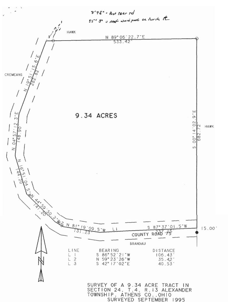
SCALE: IINCH - 100 FEET O - IRON PIN SET • - IRON PIN FOUND ASSUMED BEARINGS JOHN M. BRANNER P.S. 6805 12500 N. PEACH RIDGE ROAD ATHENS, OHIO 614-592-5778
