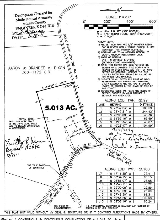
Plat of A CONTINUOUS & CONTIGUOUS COMBINATION OF A 1.041 AC. & A 3.972 AC. TRACT TO CREATE A TRACT OF 5.013 ACRES. Scale:1" = 200'
