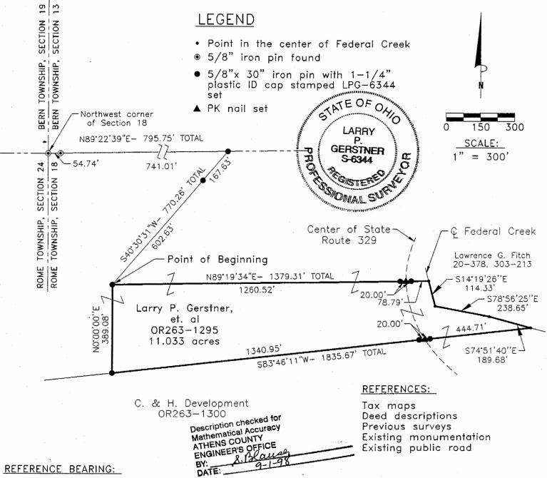
The West line of Section 18 as North 0 degrees 00 minutes 00 seconds East. Bearings are based upon an assumed meridian and are to denote angles only.
