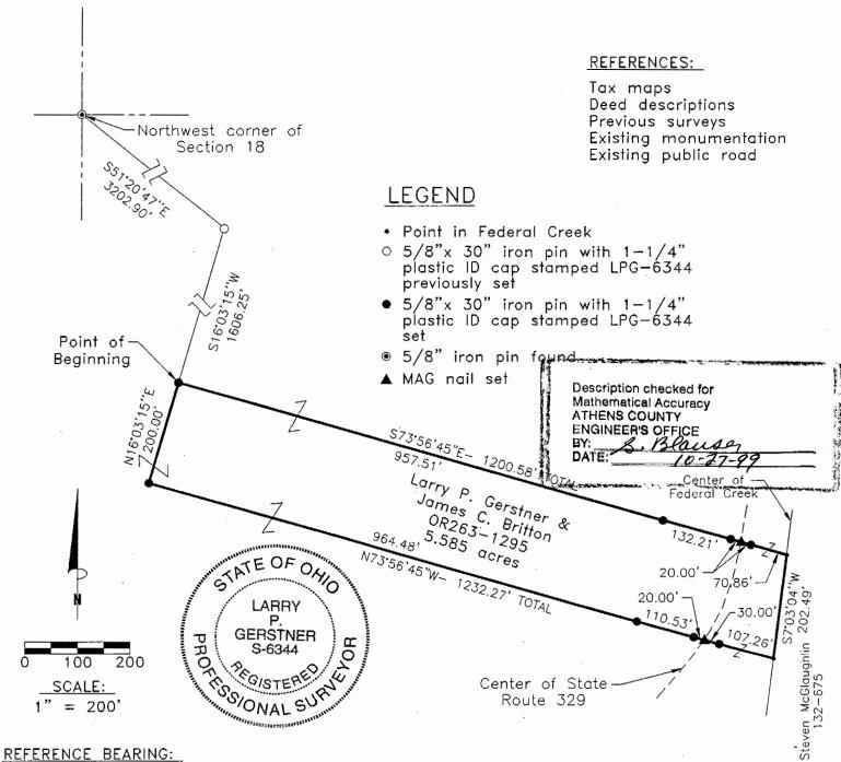
The West line of Section 18 as North 0 degrees 00 minutes 00 seconds East. Bearings are based upon an assumed meridian and are to denote angles only.
