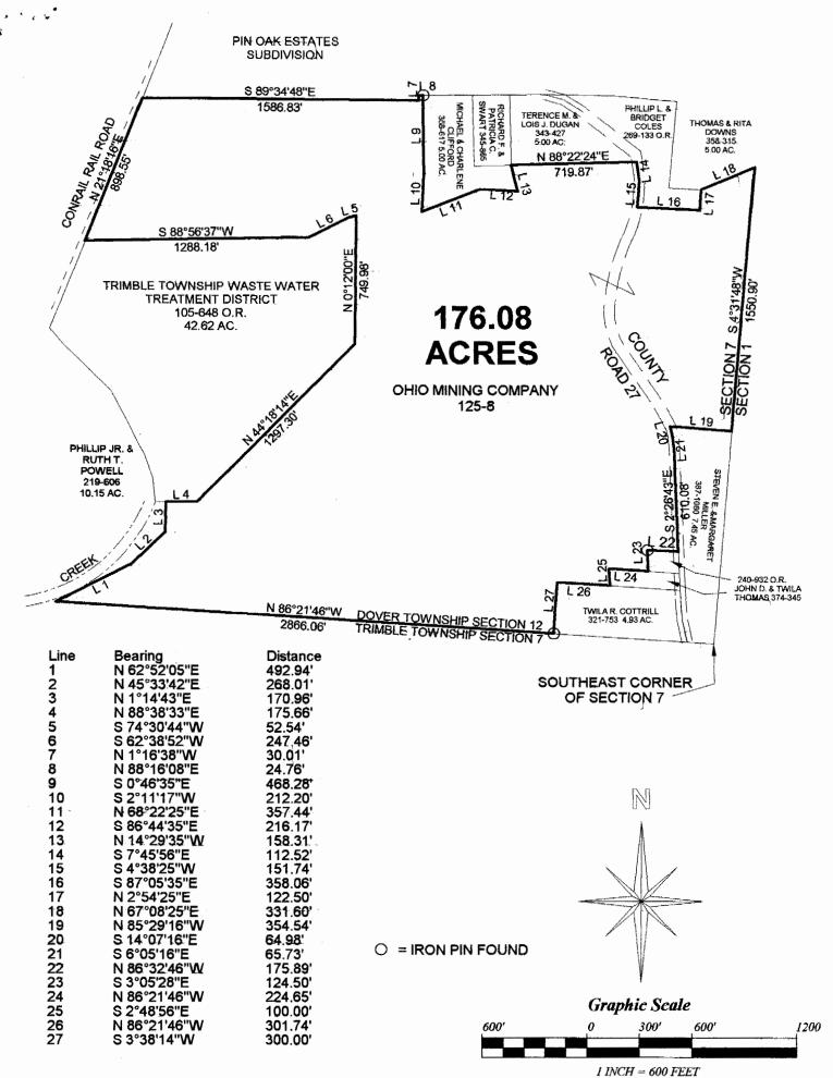
SURVEY OF A 176.08 ACRE TRACT SECTION 7, T. 11, R. 14, TRIMBLE TOWNSHIP ATHENS COUNTY, OHIO PLAT BASED ON DEEDS AND PREVIOUS SURVEYS COMPLETED JUNE 2000
