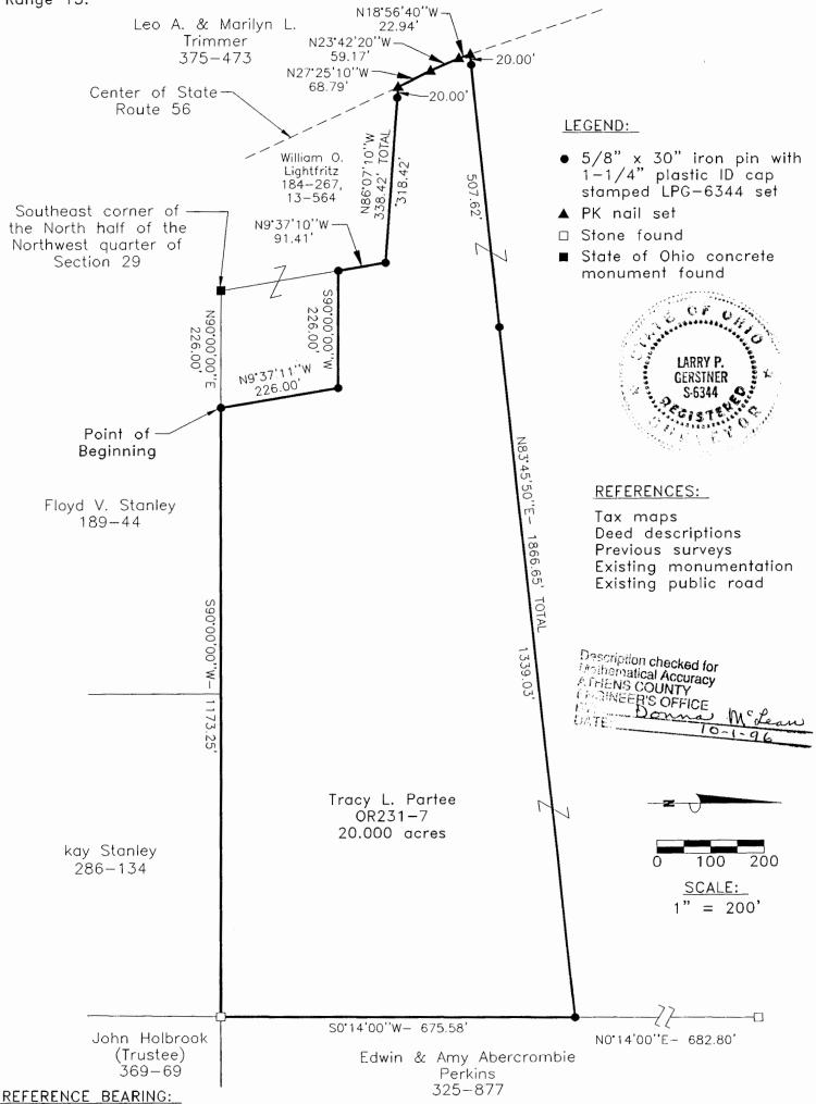
The South line of the North half of the Northwest quarter of Section 29 as North 90 degrees 00 minutes 00 seconds East. Bearings are based upon an assumed meridian and are to denote angles only.
