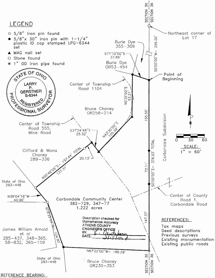
The East line of Section 36 as South 0 degrees 00 minutes 00 seconds East. Bearings are based upon an assumed meridian and are to denote angles only.
