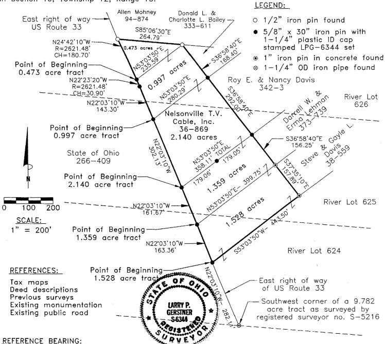
The East right of way of US Route 33 as North 22 degrees 03 minute 10 seconds West. Bearings are based upon an assumed meridian and are to denote angles only.
