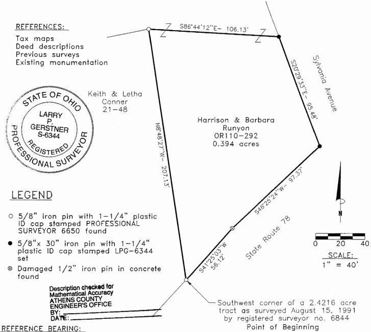
The West right of way of the old railroad as South 8 degrees 45 minutes 00 seconds East. Bearings are based upon an assumed meridian and are to denote angles only.
