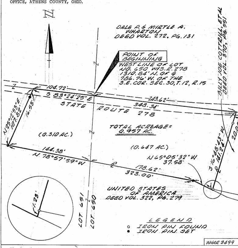
The bearing system for this plat is based on the west line of River Lot No. 650, Section 30, Township 12, Range 15 as being N 4° 10' in June of 1991 and from existing public 12" E.
