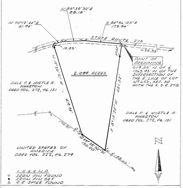
The bearing system for this plat is based on the east line of Lot No. 653, Section 30, Township 12, Range 15 as being N 7° 24' 16" E.
