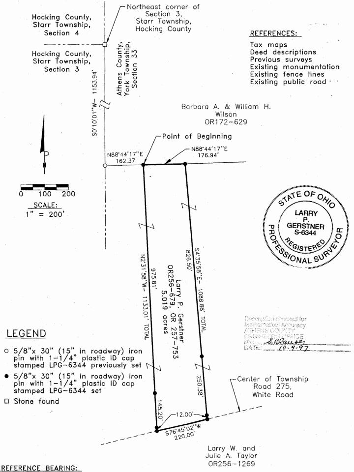
The West line of the South half of Section 33 as North 0 degrees 00 minutes 00 seconds West. Bearings are based upon an assumed meridian and are to denote angles only.
