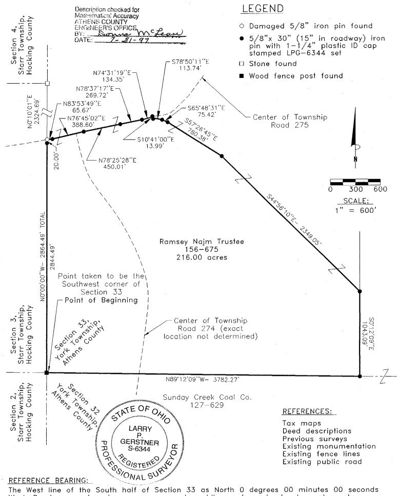
The West line of the South half of Section 33 as North 0 degrees 00 minutes 00 seconds West. Bearings are based upon an assumed meridian and are to denote angles only.
