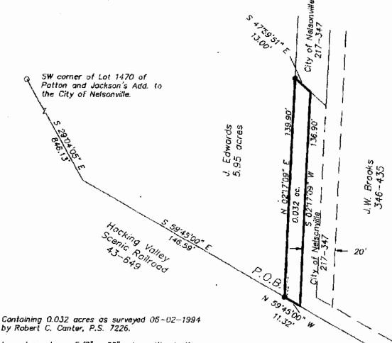
Iron pins set are 5/8" x 30" rebar with plastic cap stamped "CANTER P.S. 7226.
