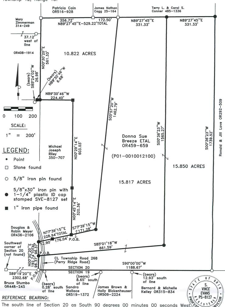
The south line of Section 20 as South 90 degrees 00 minutes 00 seconds West? Bearings are based upon an assumed meridian and are to denote angles only.
