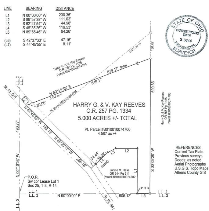
Note: Bearings are assumed and are for the determination of angles only.
