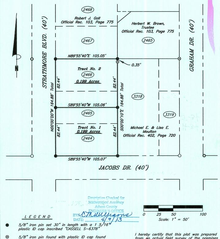
N O T E: The bearing system for this plat is based on evidence found on the East line of Strathmore Blvd. and bears N OO OO' OO" W and is for the determination of angles only.
