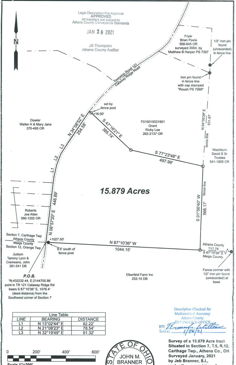
Scale 1"=200' O = Iron pin set 5/8" rebar w/ plastic ID cap = Iron pin found Bearings: N.A.D. Grid North Ref. Docs.: Tax Plats, Deeds, Existing Surveys
