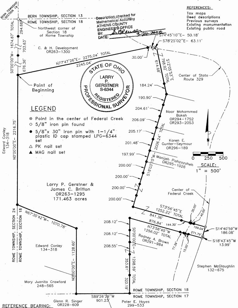
The West line of Section 18 as North 0 degrees 00 minutes 00 seconds East. Bearings are based upon an assumed meridian and are to denote angles only.
