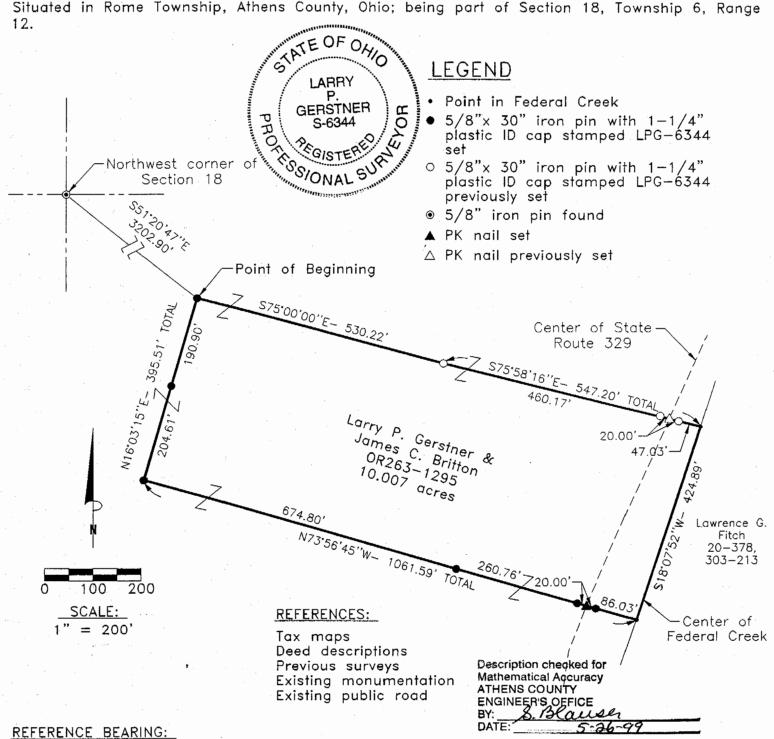
The West line of Section 18 as North 0 degrees 00 minutes 00 seconds East. Bearings are based upon an assumed meridian and are to denote angles only.
