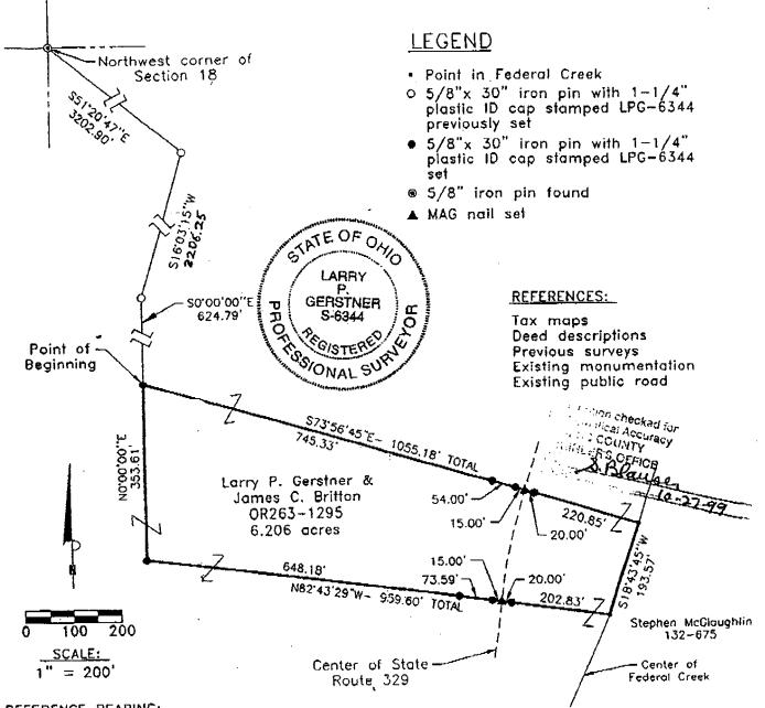
REFERENCE BEARING: The West line of Section 18 as North 0 degrees 00 minutes 00 seconds East. Bearings are based upon an assumed meridian and are to denote angles only.
