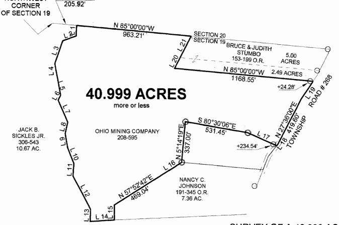
Line Bearing S 3°00'00"W Distance 88.44 117.48 S 71°00'00"W S 19°30'00"W 199.32 S 1°00'00"E 126.06 S 19°00'00"E 142.56 S 28°30'00"W 44.88 S 24°00'00"E 201.30 S 13°00'00"W 95.70 120.78 S 10°00'00"E S 22°00'00"E 141,24 102.30 11 S 4°00'00"W 12 13 14 15 S 28°05'26"E 314.14 S 2°14'33"W 98.301 N 86°10'13"E 203.70 N 0°49'47"W 123.81 16 17 N 58°06'34"E 200.17 S 66°07'43"E 264.54 19.52' 18 N 34°45'13"E 19 20 N 34°18'00"E 176.00 100.00 N 27°14'30"E 21 N 27°14'29"E 200.001
