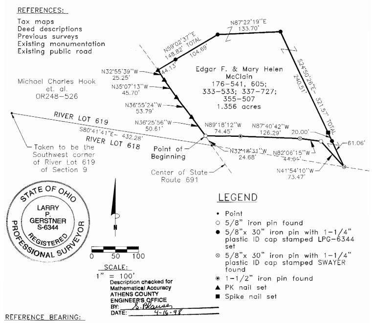
The South line of River Lot 619 as South 80 degrees 41 minutes 41 seconds East. Bearings are based upon an assumed meridian and are to denote angles only.
